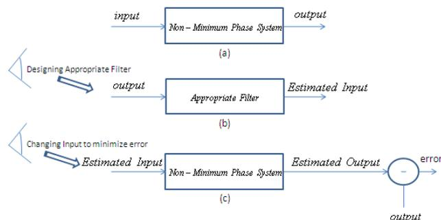
Fig1: a) Non-minimum phase system. b) Viewpoint of previous works in deconvolution problem that causes to design appropriate filter reach to input signal. c) Viewpoint of proposed method which.
