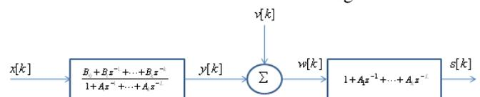
Fig11: Convert ARMA model to MA model
