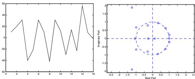
Fig7: Left: the impulse response of system, Right: pole-zero plot
