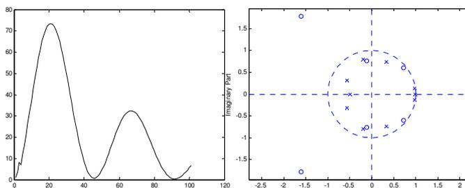
Fig12: Left: the impulse response of system, Right: pole-zero plot
